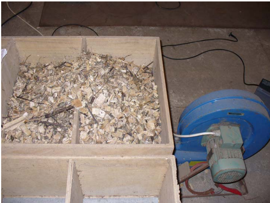
Fig2. Containers to allow air to be blown through the samples.
