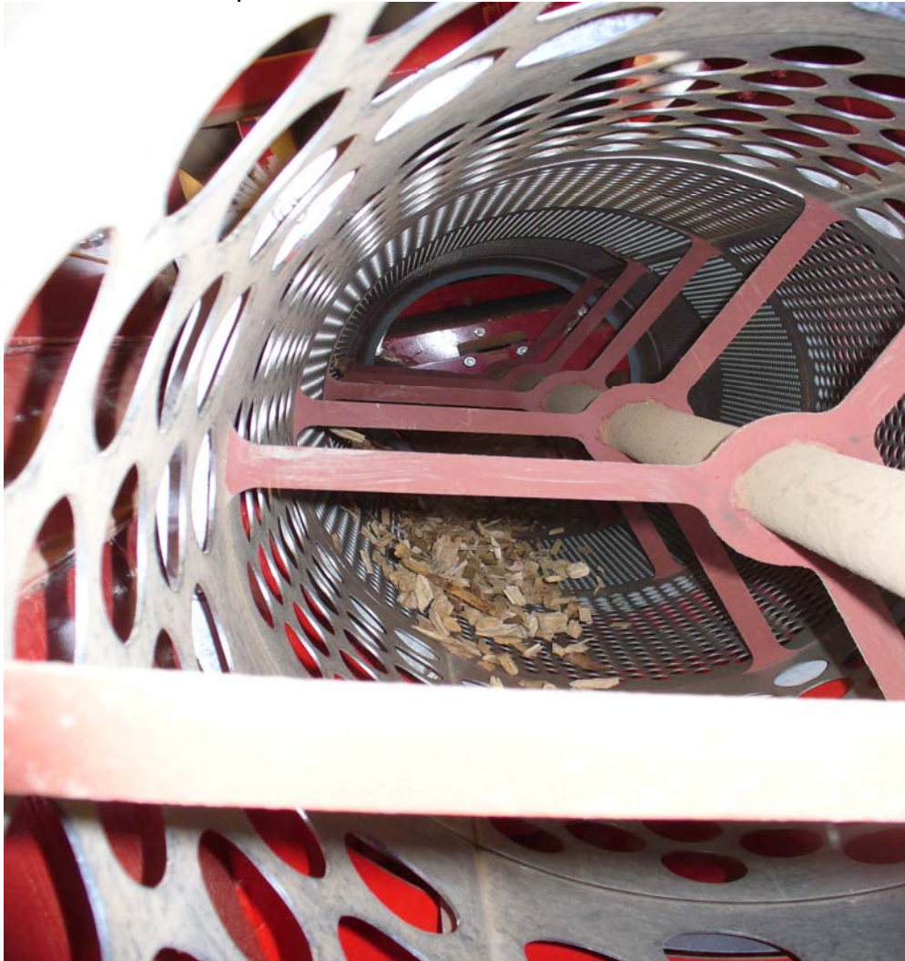
Fig6. Wood chip in rotating in particle size drum, showing particles passing over smaller with 3mm holes, 8mm, 16mm, 45mm, to mesh of 63mm.
